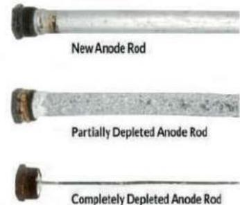
Failure to inspect the anode rod at least once a year could cause the tank to fail and leak. This condition is not covered under the manufacturer warranty.
