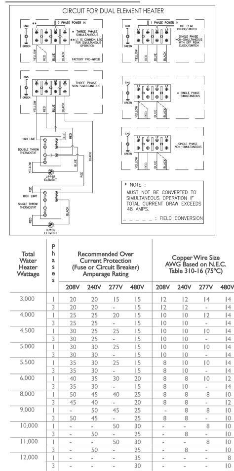
AUTION: If wiring from our fuse box or circuit breaker box was aluminium for your old water heater, replace it with copper wire. If you wish to reuse the existing aluminium wire, have the connection at the water heater made by a competent electrician.
