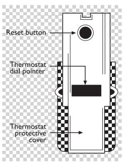
Type 59T thermostat and protective cover The water heater is equipped with combination thermostat
