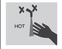
Water temperature over 125° F can cause severe burns instantly or death from scalds.
