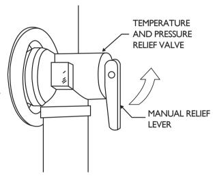
Figure II DISCHARGE LINE TO DRAIN
