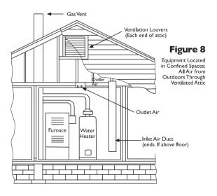
I. When communicating with the outdoors through horizontal ducts, each duct openin shall have a minimum free area of I square inch per 2,000 BTU per hour of total input rating of all equipment in the enclosure. (figure9)
