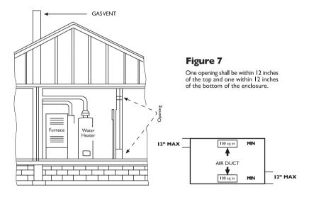
When communicating with the outdoors through vertical ducts, each opening shall have a minimum free area of I square inch per 4,000 BTU per hour of total input rating of all equipment in the enclosure. (Figure 8)
