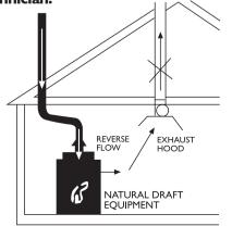
POTENTIAL HAZARDOUS DOWNDRAFT OPERATION . EXHAUST FANS . VENTILATION SYSTEM . CLOTHES DRYERS . FIREPLACES . OTHERS After completing all gas connections, check each gas connection and fitting for leaks. Use a soap and water solution or a commercial leak detector fluid. NEVER USE MATCHES OR OPEN FLAME WHEN CHECKING FOR GAS LEAKS.
